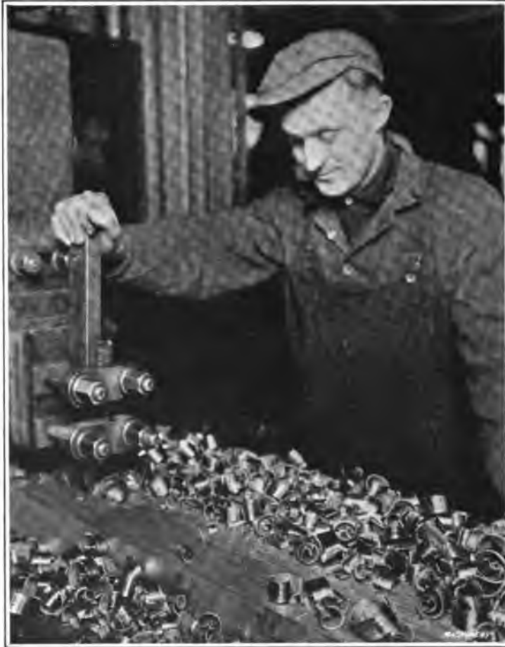
Fig. 2. Planing with a High-speed Steel Tool
